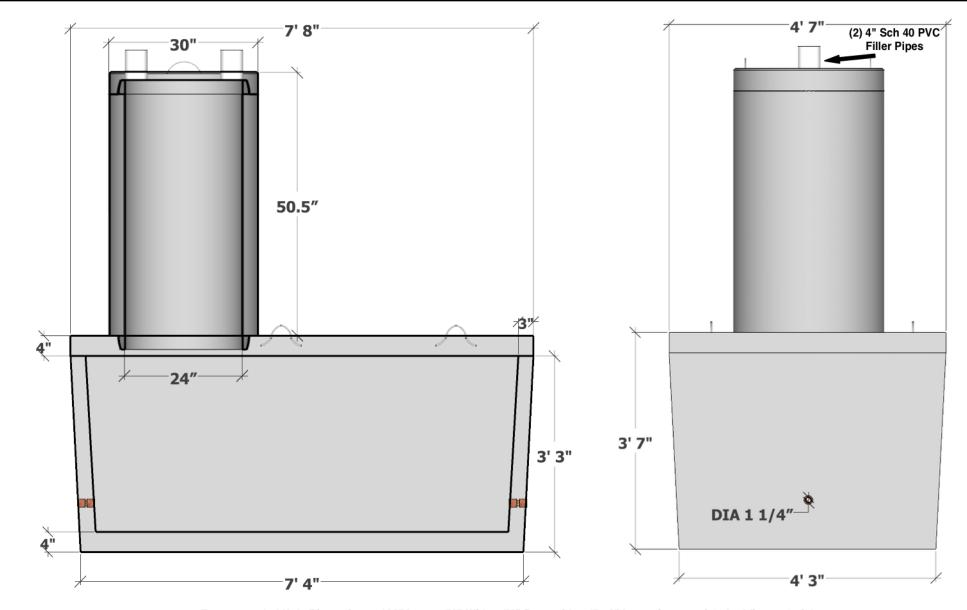
Recommended Hole Dimensions - 108" Long x 72" Wide x 78" Deep with a 4" - 6" base of appropriate bedding material
